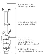
Distance between hydraulic access fittings should be minimum 300 mm center-to-center.
